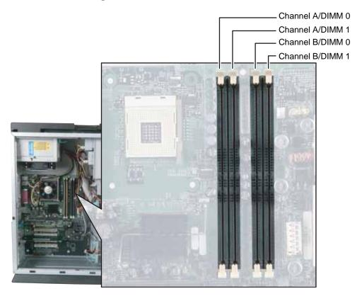
**5** Align the notches on the new DIMM with the notches on the memory module bank and press the module firmly into the bank. The tabs on the sides of the memory module should secure the memory module automatically. When the module is secure, you hear a click.
